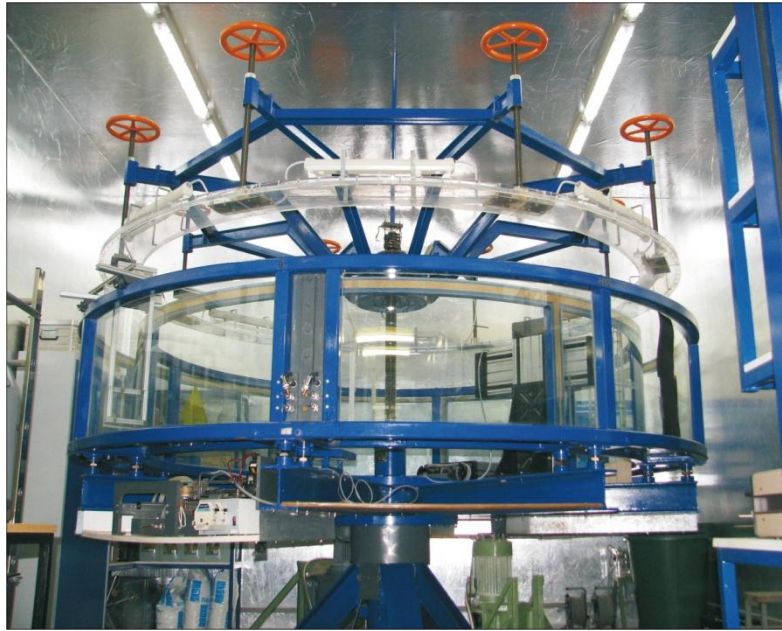
Figure 1.11 Annular flume located at the Institute of Hydraulic Engineering and Water Resources Management, RWTH Aachen University, Germany (Photograph provided by Dipl.-Ing. Catrina Cofalla).
